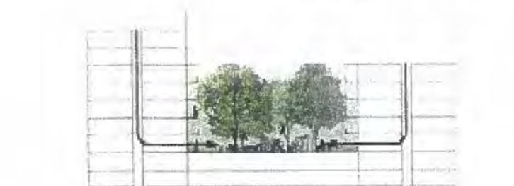
sec. A - potential section through a typical housing block showing access and lines of sight to play area
